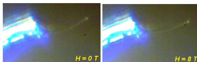
Figure 2 Giant magnetic-field-controlled bending strain of composite microactuator in Bitter coil at constant temperature. The composite is bent in zero field and strained almost completely at \mu_0 H = 8 T due to interaction of the elastic and prestrained active layers with SME.
