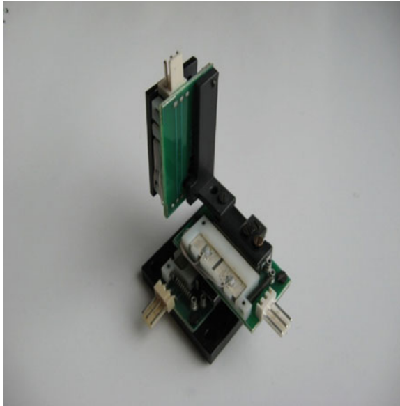
Fig. 3 3-D nanomanipulation system based on innovative piezomotor is developed with parameters as follows: motion range—15 mm, minimal step—10 nm, thermal drift <5 nm/h at 20 °C; speed of linear motion along any of 3 coordinates: 20–20 mm/s [83–92]
