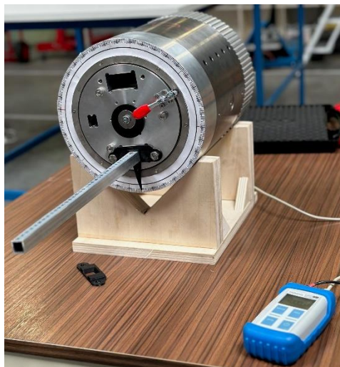
Figure 3 : Measurement of the magnetic field homogeneity at different measurement points
