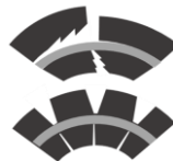
Schematic illustration of unstructured and structured electrodes after winding at small radii
