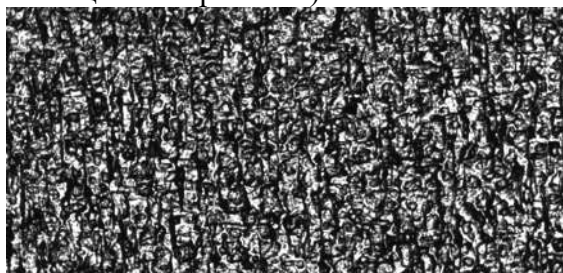
Fig. 2. The section of the GaAs plate after etching in the melt of anhydrous KOH
