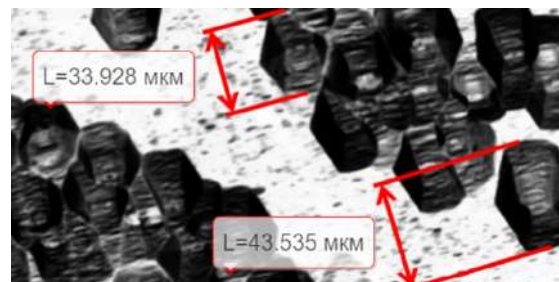
Fig. 5. Etching pits of a plate with an activated surface after etching in a NaOH·H 2 O melt
