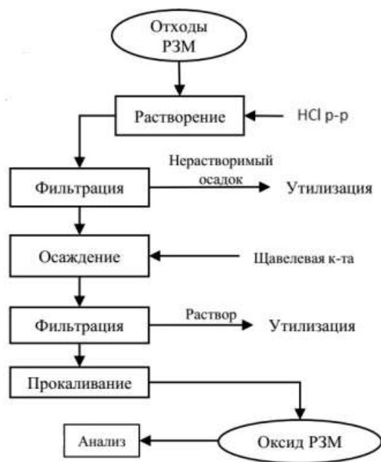
Fig. 2. REM waste recycling scheme
