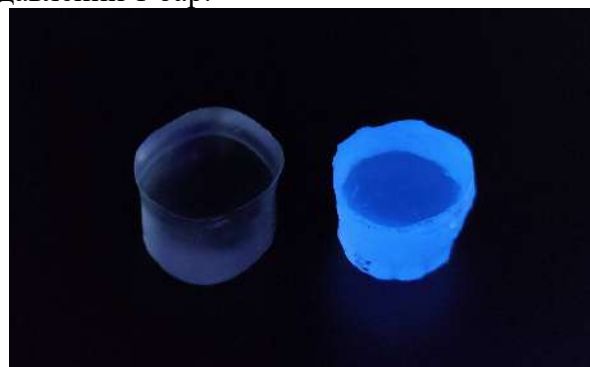
Fig. 1. Luminescence of CsI:Yb 2+ crystal (right) compared to a pure CsI crystal (left) under 395 nm excitation
