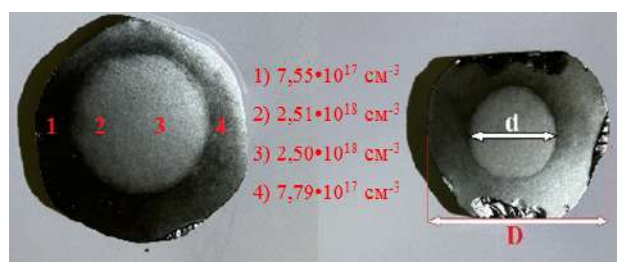
Fig. 2. Concentration heterogeneity in InSb (111)
