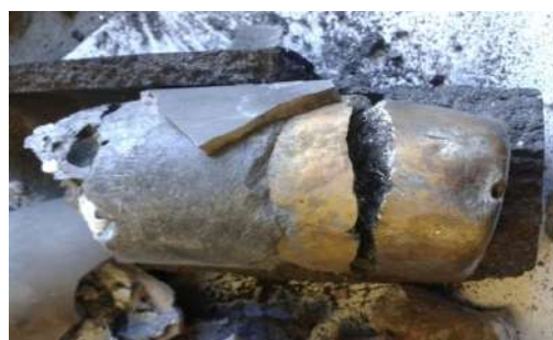
Fig. 2. Products of co-reduction of aluminum oxides after melting the charge in a corundum crucible in a GM 16 440 induction furnace with a capacity of 15 kW. Metal composition, %: Zr – 44.36, Al – 48.06, Mo – 3.9, Ti – 4.12, N – 0.009, O – 0.09
