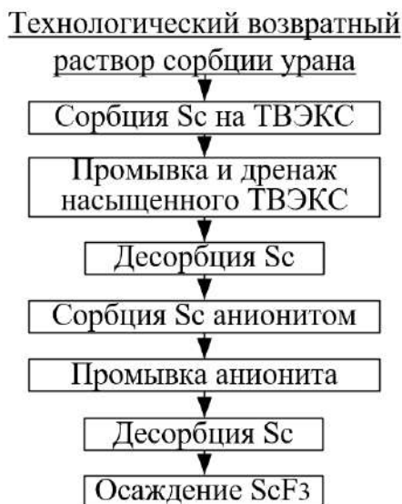
Fig. 1. Principal technological scheme for production of conditioned scandium trifluoride
