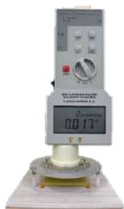
Fig. 1. Surface potential measurement process \varphi
