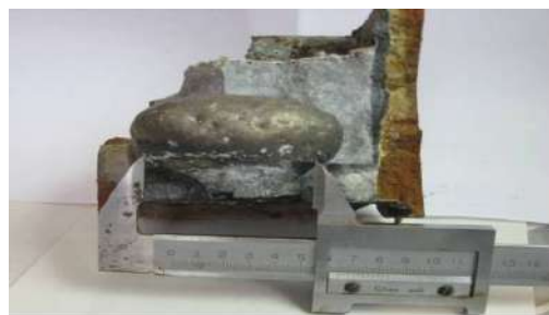
Fig. 1. View of the Al-60%Ti alloy ingot and slag after melting in a two-electrode electric arc furnace
