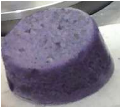
Fig. 1. Type of fuel composition 72,2 mol. % LiF – 26,7 mol. % BeF 2 – 1 mol.% Pu(Am)F 3
